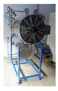
• SS Cylindrical Autoclave which is of high premium quality and can be availed by us only. Our cylindrical autoclave is incorporated with water level indicator, vacuum breaker, automatic pressure control switch, and steam trap. We are also well known cylindrical autoclave manufacturers in India.
